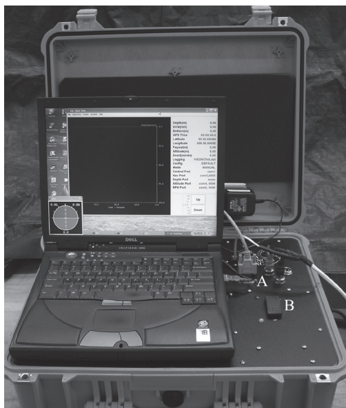
Fig. 2. The Control and Power Distribution module fits inside a single Pelican case. AC-to-DC power converters and data transmission hardware are secured to the case underneath the laptop. Also visible are (A) the external data and power connections to the tow cable and (B) the manual rocker switch for overriding the wing angle set by the computer.
